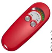
A UVA Meter can quickly and clearly show the condition and quality of the UV output of existing fluorescent tubes in a fly trap, showing whether they are working at peak performance, in need of replacement or beyond useful life.
